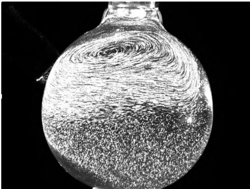
Figure 3.10: Pathline visualization from 10- Celsius temperature difference (upper heating) These 100 images were taken from 5 mins to 5 mins and 10 secs. Note that most of the flow behavior was happening on the top part of the eye model.
