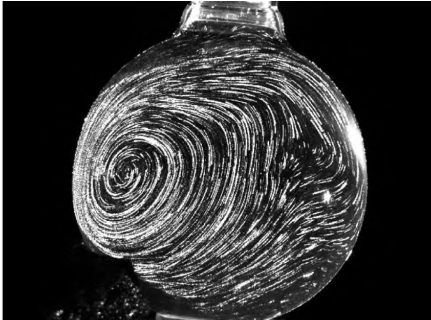
Figure 3.9: Pathline visualization from 10-celsius temperature difference (lower heating) These 100 images were taken from 5 mins to 5 mins and 10 secs. Note that circulations were fully activated across all regions in the eye model.
