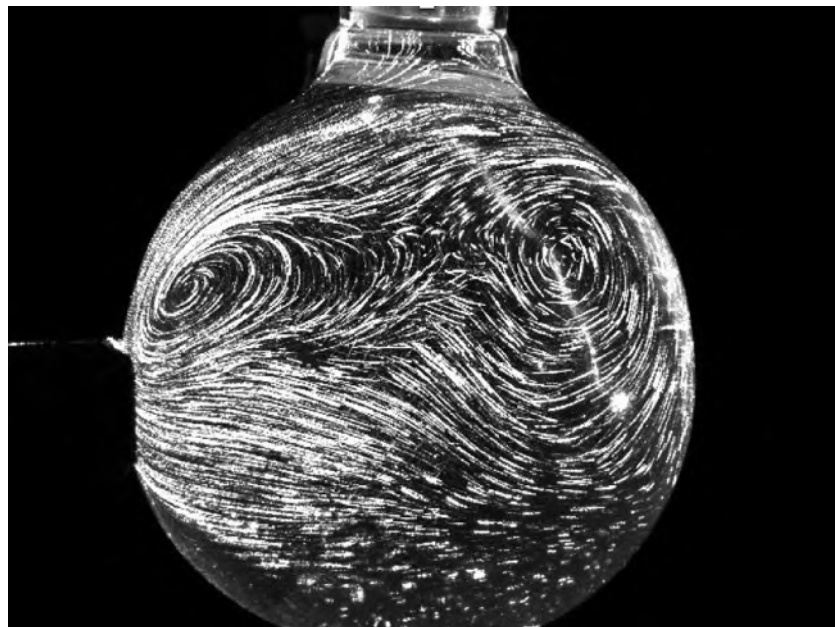
Figure 3.8: Pathline visualization from 10-celsius temperature difference (center heating) These 100 images were taken from 5 mins to 5 mins and 10 secs. Note that the flow was stronger compared with the one in Figure 3.7a, although circulation was relatively weak at the very bottom of the eye model.
