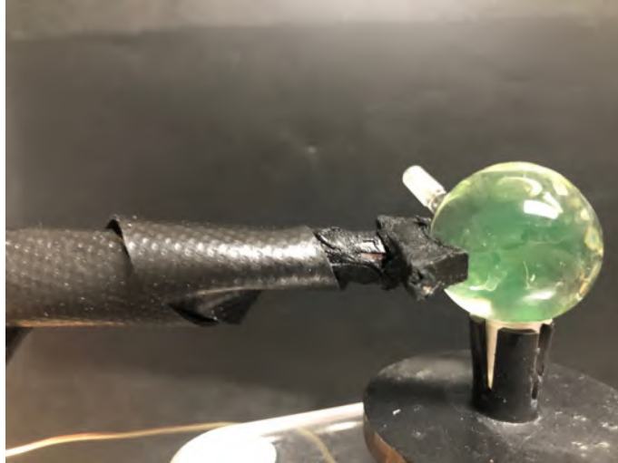
Figure 3.4: Heating element at the “center” heating location
